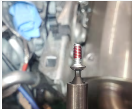
Stainless steel screw with sealant
