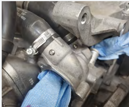
Screw installed in housing to affix the coolant pipe
