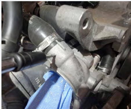
Tapping the screw hole in the housing
