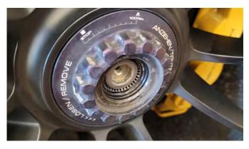
Internal lock in proper place. A tool is included with your vehicle to facilitate this.
