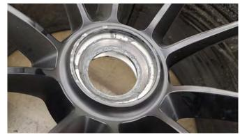
The dark gray line is the contact patch on the wheel from the lock. This should be at least 10-15mm in width
